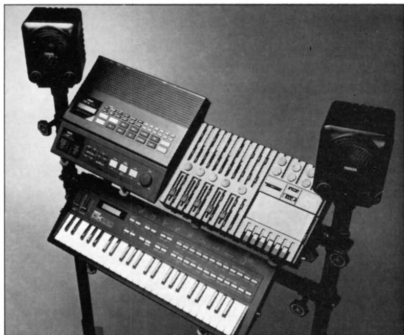
*The System 100: QX21 digital sequence programmer, RX21 digital rhythm programmer, DX100 FM digital synthesizer, MT1X Multi-track cassette recorder, and two KS10 keyboard speakers, all mounted on an ST100 stand.*
