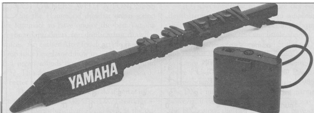
**T**HE WX7 is a MIDI wind controller designed for use by saxophone players (and those who play other woodwind instruments). Like other MIDI controllers, the WX7 makes no sound by itself—it must be connected to a MIDI synthesizer or tone generator. The tone generator produces the sound, and the WX7 controls and shapes the sound produced by the tone generator.
