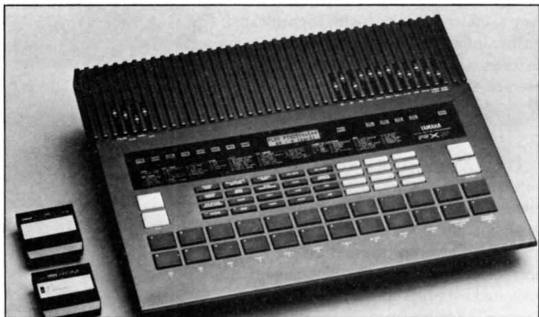
the MIDI Pitch mode allows you to access up to 16 different sounds simultaneously and “play” them across 5 octaves of pitch from a MIDI keyboard (such as the DX7 II).
